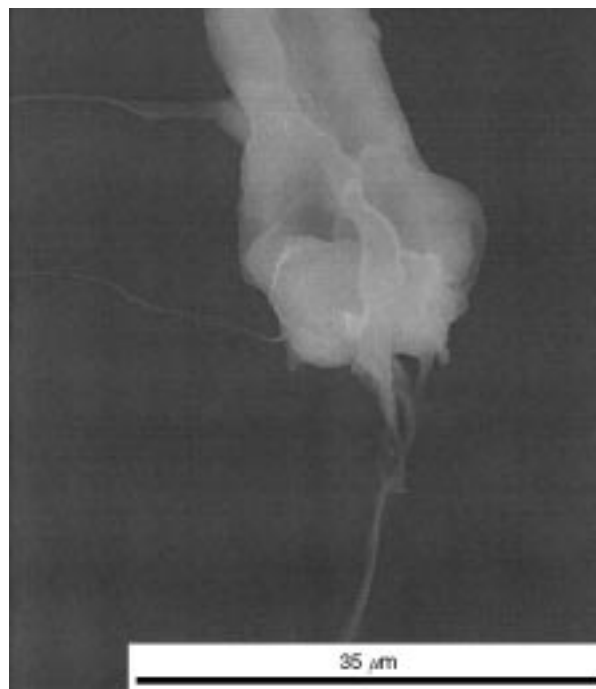
Figure 6 Melt damage—UHMWPE fiber.
