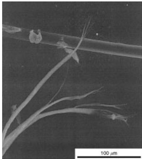
Figure 4 Fibrillation of aramid fibers.
